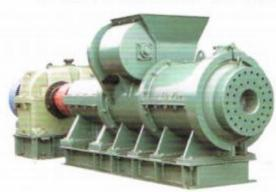
technology that extrusion fuel coal powder into a certain intensity of coal rod and sent it into gasification furnace for combustion instead of the lump coal. It can make full use of coal power and reduce the cost fuel.
