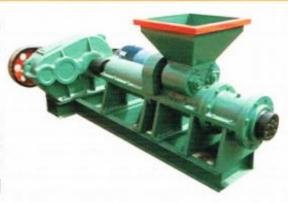
Coal rod extruder is the main equipment in the shaping process of fuel, It is a new
